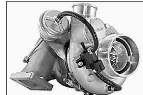
Patent-pending ceramic ball bearings increase thrust capacity and durability while reducing frictional losses, all for a 3 to 4 percent improvement in turbine efficiency at low expansion ratios.
